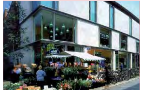
Large floor plate uses such as supermarkets must be carefully designed to provide active frontages: glazing allows views in, additional uses such as cafes and small shops create activity, and otherwise blank frontages can be screened by other uses such as residential.
