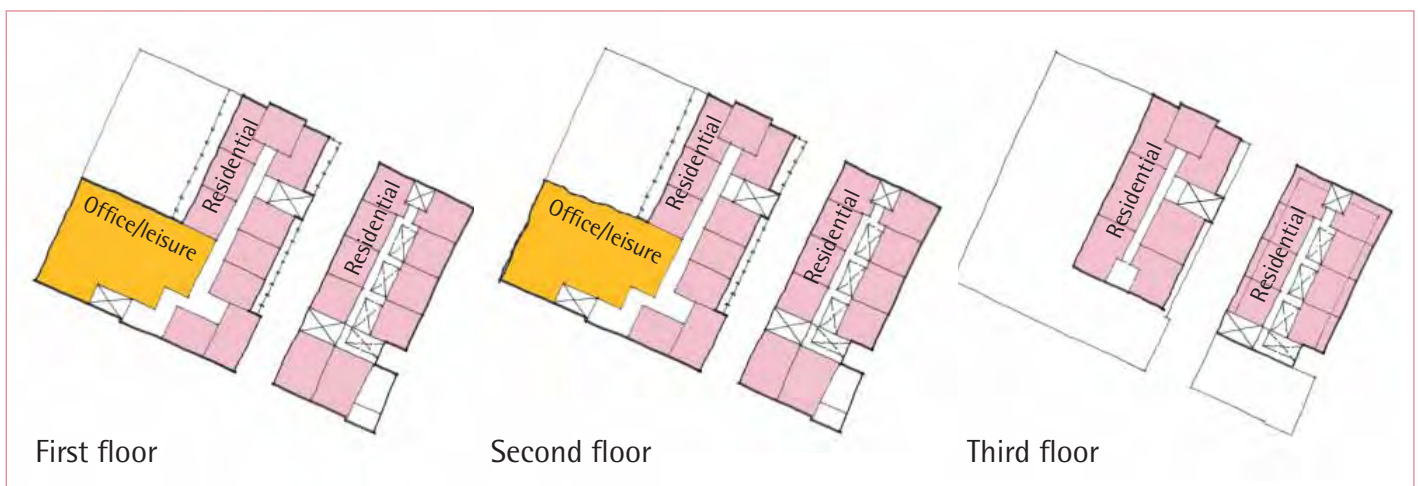
Figure 4.4: Sketch plans showing how upper floor uses within both new buildings could be organised.
